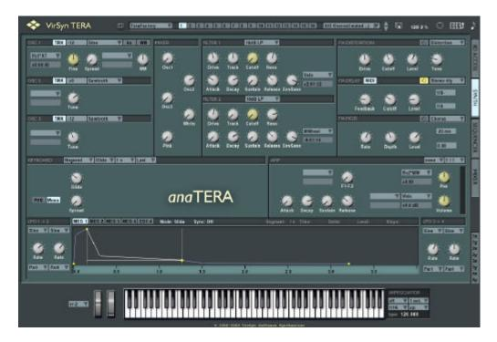
This synth is an enhanced classically modelled analogue synth. The 3 main oscillators of TERA are feeding the 2 standard multimode filters in parallel. The output of both filter modules can then be morphed for the resulting output. But keep in mind that despite this simple base structure you can do much more than with any previously existing analogue synths due to the multi-segment envelopes and the possibility to specify your own waveforms for each oscillator.
